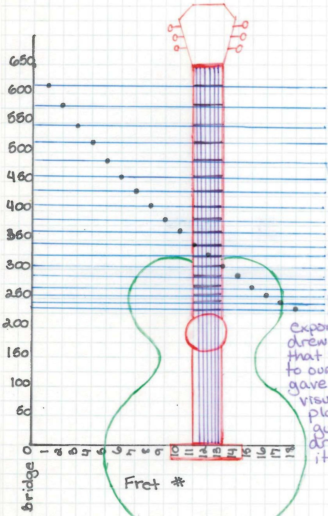
This is a visual representation of how we were able to calculate the fret positions on our guitar. As the note frequencies increased exponentially, the fret positioning decreased exponentially. We drew straight lines that were parallel to our x-axis. This gave us a clear visual of the fret placement. The guitar was then drawn to show its appearance.
